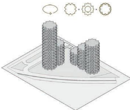
Sketch 05: Exploring the rotation and variation of the traditional rectangular shape of the building, we came out with a rich yet simple and modular shape. The rotation of the module by 45° at every floor creates free corners were the private terraces of the different housing units could be placed.
